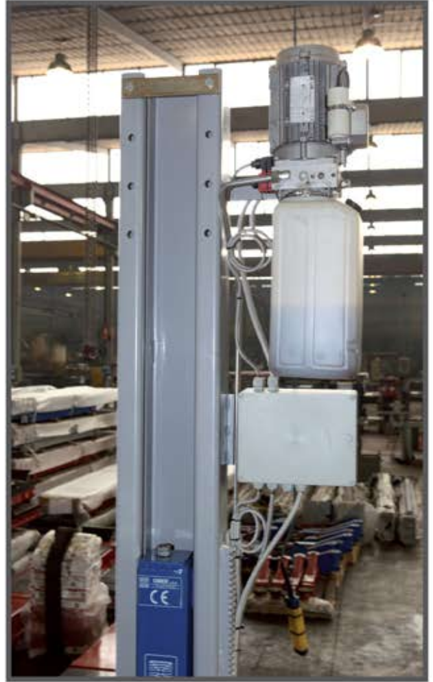
The compactness of the electro-hydraulic assembly and the electrical panel - located at the top of the left hand column - ensures the utmost efficiency in minimal space, thus ensuring unhindered parking of the car.
