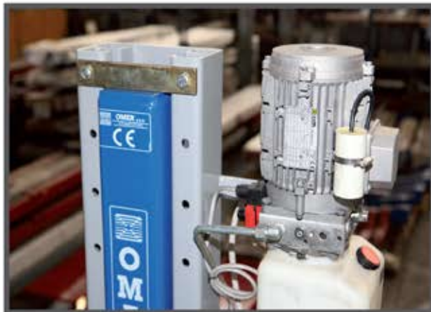
The vertical lifting height of the platform is set during the initial installation by means of locking steel plates mounted at the top of the columns, thus guaranteeing safety and
