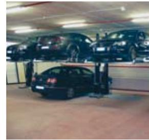
The system is suitable also for installations in series as the base of the plant is crossable and it can be fitted to the floor.
