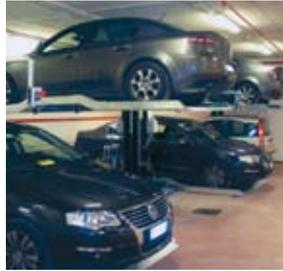
System IP1-ML does not have lifting ropes or chains and practically does not need maintenance.
