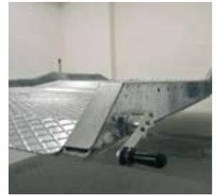
*A mechanical block assures the platform in raised position also in case of pressure drop of the hydraulic system. In order to lower the platform it is necessary to unlock the mechanical block through the manual lever first.*
