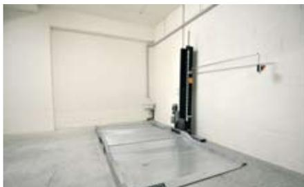
*Inner sight of a garage that has the IP1-ML system installed with lowered platform. The column can be realized on the right or left side. The height under the platform is adjustable from 155 cm to 200 cm in order to park any type of car.*
